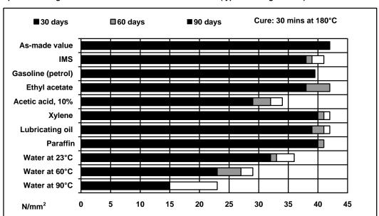
Lap shear strength after immersion in various media at 23°C (typical average values)
