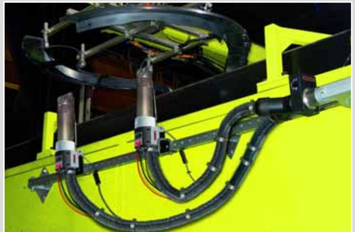
The plastic parts are deburred with a jet of hot-air following the injection moulding process.
