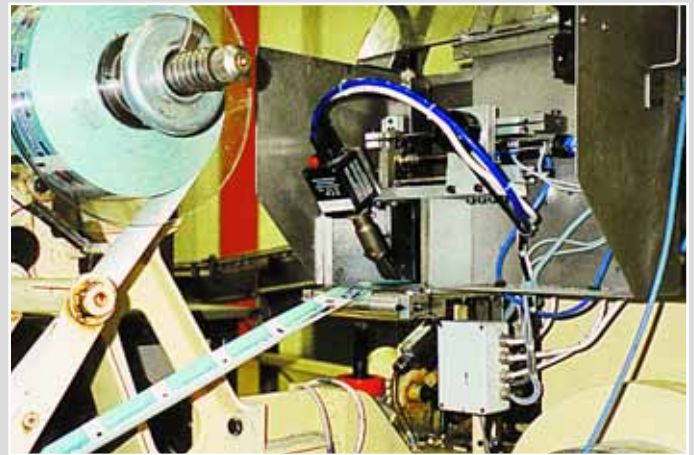
Air heater and blower for drying labels. Fast drying allows a high throughput speeds.
