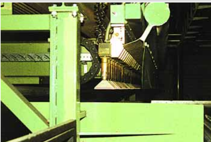
64 air heaters burn marking lines on insulating plates in a crosswise pattern without using paint.
