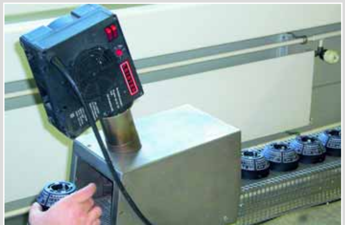
A hot-air blower with spoon reflector brands the paint after pad printing and so makes it scratch resistant.
