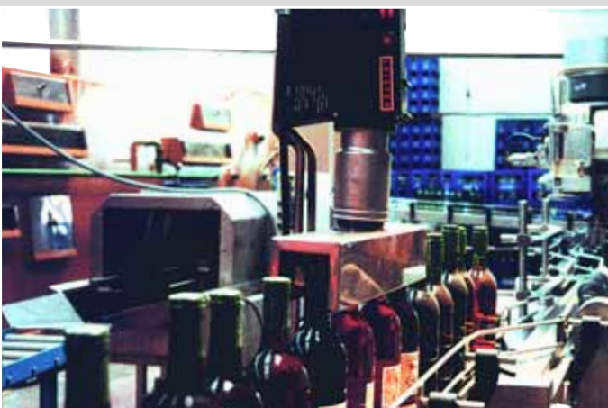
Shrinking capsules with a hot-air blower and push-on spoon reflector.
