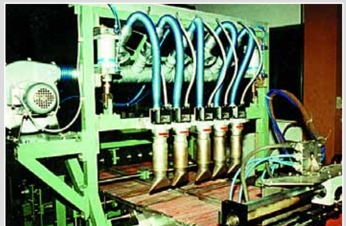
Blower and air heater soldering cooling fins. With hot-air this work can be performed without mechanical distortion.
