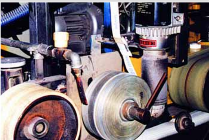
Air heater with blower welding a PVC continuous hose.
