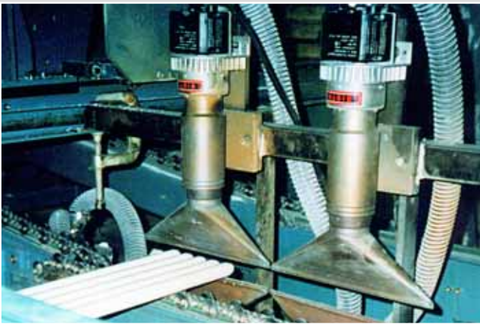
A Heater and blower used to heat the ends of fluorescent tubes. This removes the coating before gluing.
