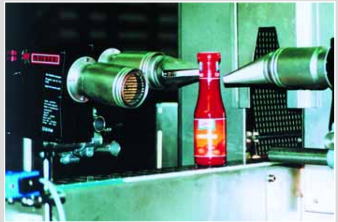
Three hot-air blowers shrinking shrink caps onto bottles.
