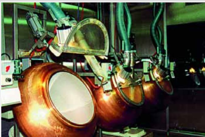
Drying and smoothing pills, dragées, sweets and their coatings with air heaters and blowers. Regulated air temperature with Leister controllers.
