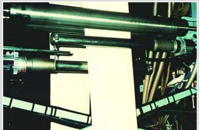
Preheating a paper strip prior to printing with space-saving long tube nozzles.
