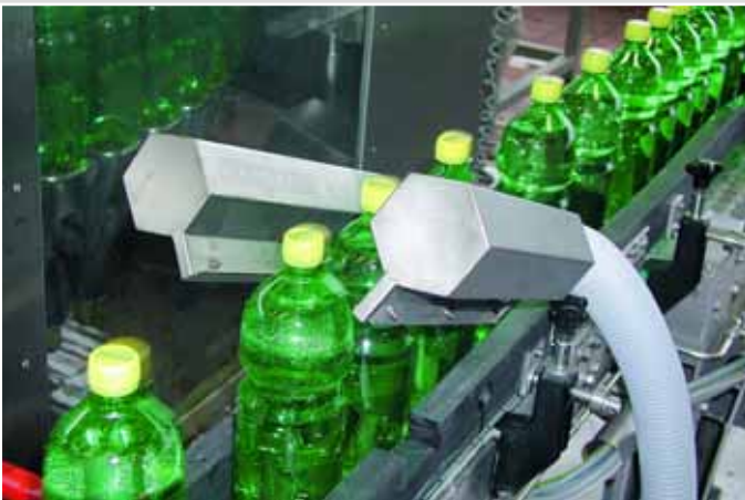
The combination of blow-off nozzles and blowers allows fast and efficient drying of beverage bottles.
