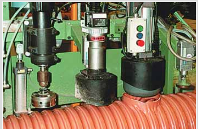
Air heaters and blowers performing partial heating of a PVC pipe for subsequent shaping of the branches.
