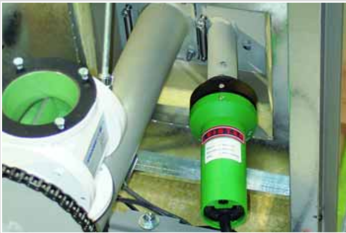
Igniting wood pellets or wood chips with the Leister TRIAC S ECONOMY.
