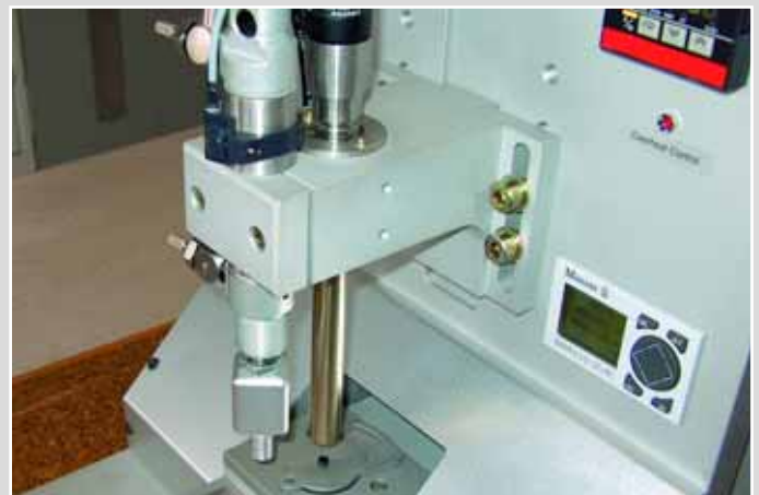
LE MINI SENSOR air heater warms a plastic rivet, which is then formed with a cold die.
