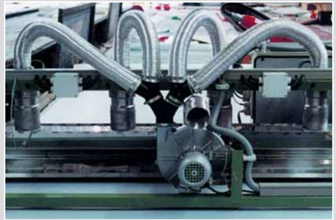
A blower supplies four air heaters printing ink on textiles.
