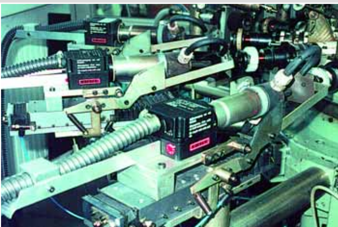
Melting of self-bonding wire on coils for transformers and motor windings is carried out in the winding process with hot-air.
