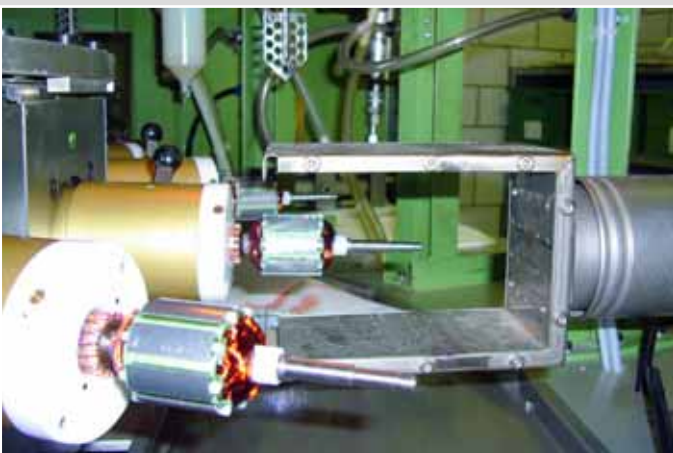
Drying of wet rotors with hot-air and sieve reflector.
