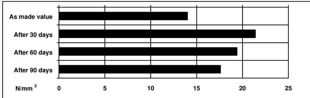
**Lap shear strength versus heat ageing (ISO 4587) (typical average values)**
