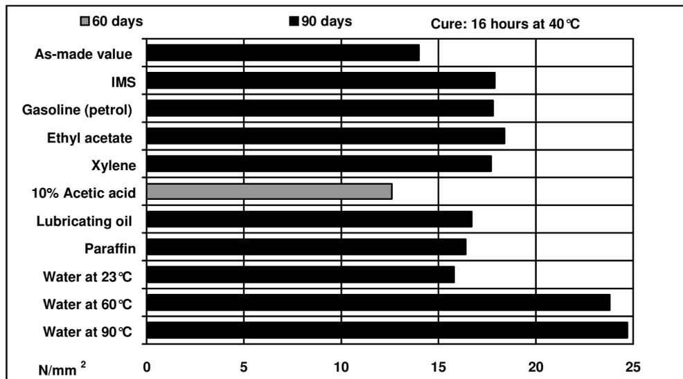
**Lap shear strength versus tropical weathering (ISO 4587) (typical average values)**
