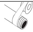
Holding the reel as shown in the diagram above avoids the need to unroll too much tape when applying it.
