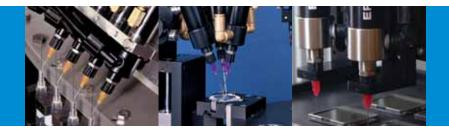
The complete system includes the 741V dispense valve, ValveMate  $^{\scriptscriptstyle \rm M}$  8000 controller, the fluid reservoir and dispense tip.
