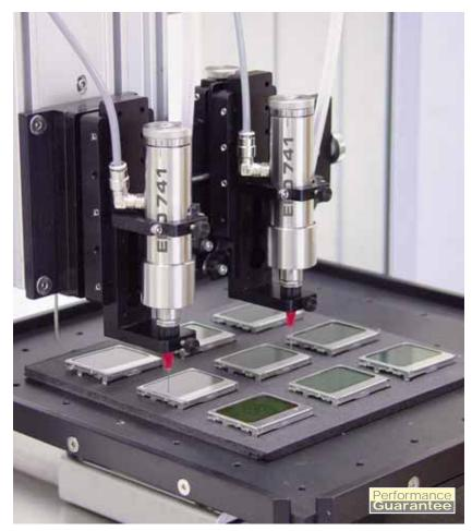
"We needed something that was accurate, repeatable and easily validated, and we found it. We're very pleased with the accuracy of these systems, particularly with their repeatability." Retractable Technologies, Inc. The 741V Series valve design applies low viscosity assembly fluids with accurate, extremely close repeat deposit control.
